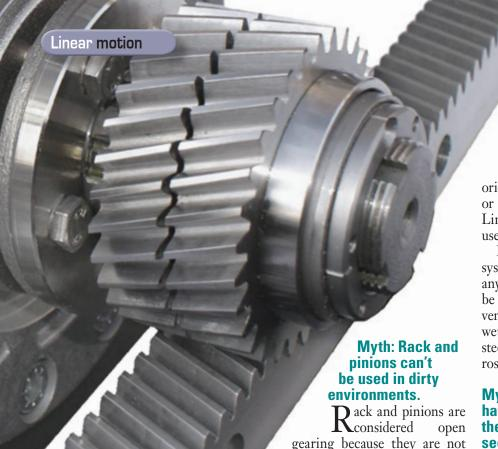
orienting the rack teeth on their side or facing down can minimize this. Linear bellows or covers can also be used to protect the drive.
