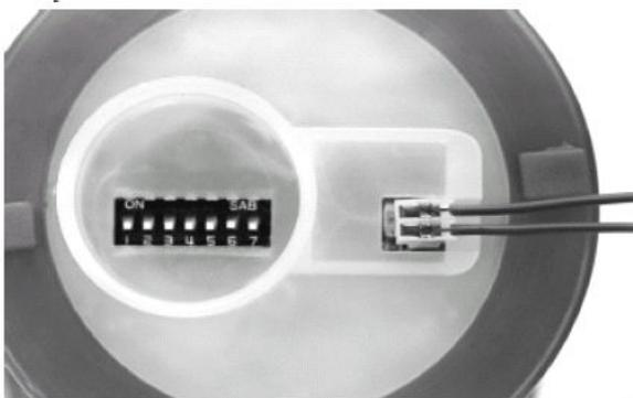
Setting same as so far. Extend contact cable and connect to limit switch or contactor with floating contact. No external power supply required.
