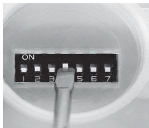
Any dosage required can be set via DIP switch combinations
