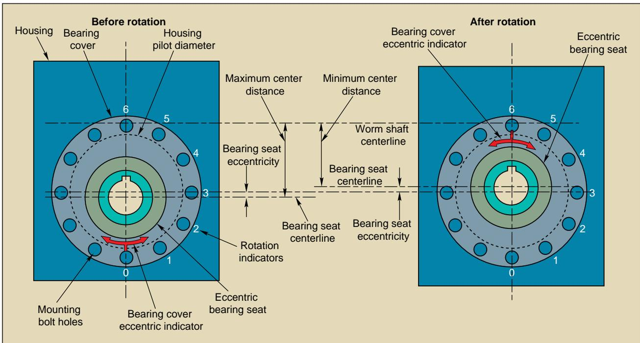
**Figure 3 — Bearing covers move the worm gear shaft up to reduce backlash. For lower backlash, rotate each cover so its indicator moves from its original position to the next higher position on the housing. This moves the worm gear up into a tighter mesh with the worm, thus minimizing backlash between them.**
