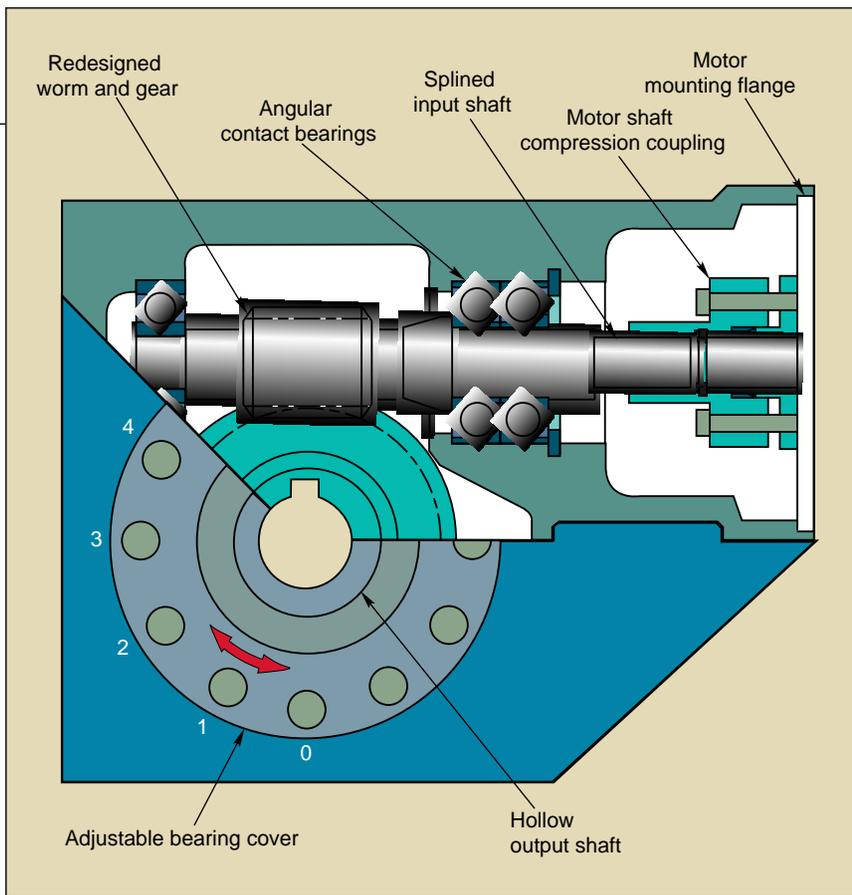
**Figure 4** — To reduce backlash, new gearhead combines improved gear tooth profiles, adjustable eccentric bearing covers, and precision angular contact bearings. Other features include an input mounting flange for most servomotor types and a hollow output shaft to accommodate various driven load connections.
